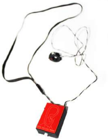
Rode Oortjes Meter 2014, Black 3D printed box (45x30x25mm) + Red laser-etched Plexiglas + PCB board + components + battery + black ear clip consisting of two glued 3D printed forms with RGB-LED and (orange) thermistor + 4 thin braided electrical wires, 53 x 30 x 25 mm, device that arousal measures on the basis of the temperature of the ear.
