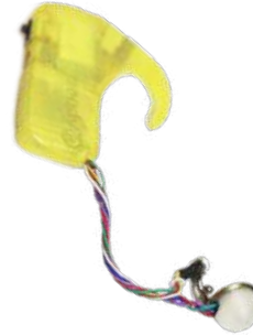
MOODY® 1.0 2018 - Excitement Calculator: This jewelry shows the excitement-color (an rgb-light) continuously by measuring the temperature of the ear constantly. The device connects with server. The new version is smaller (fixed behind the ear and clipped on ear) and can transmit data via BLE using a ESP32. Components: ESP32, Li-battery, tiny wires, infra-red temp sensor, rgb-led, on/off switch, earclip and 3D-printed case.
