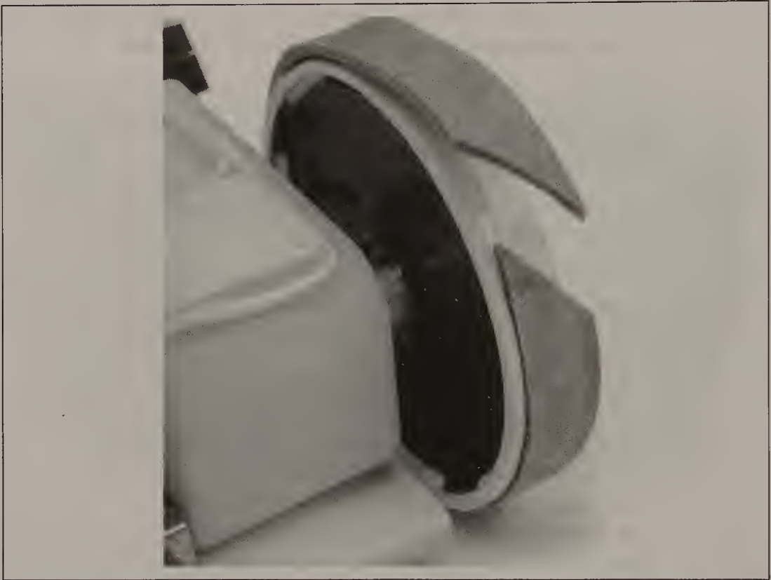
Figure 12-36 Gluing rubber bands to the wheels for better traction
