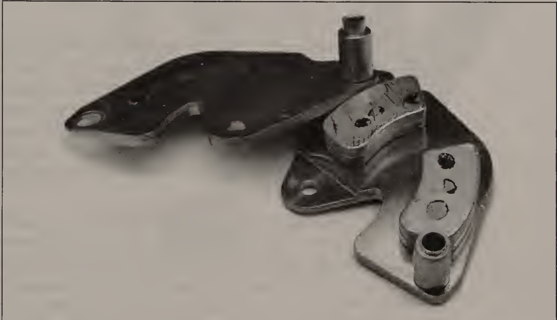
Figure 11-5 Supermagnets, found sandwiched between two spacer plates in a dead hard drive
