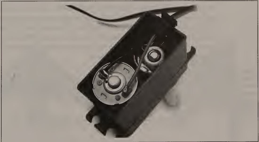
Figure 13-11 Wiring up servo motor leads and laying down the wire with the rubber grommet
