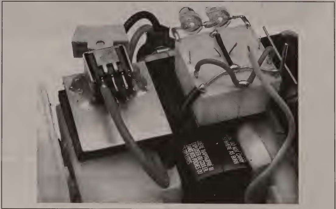
Figure 12-32 Red to switch, black to relay brick
