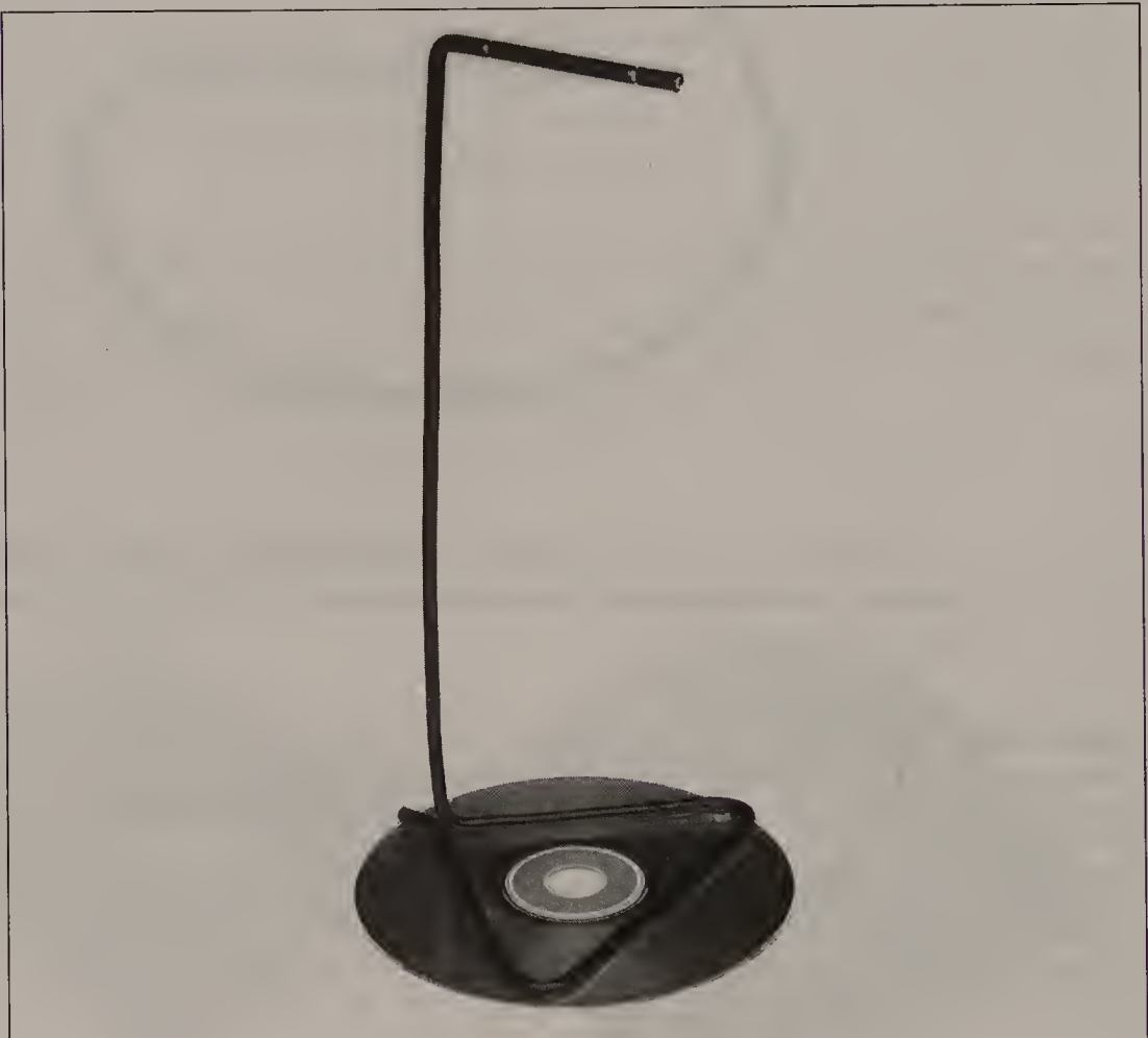
Figure II-29 Wire support arm glued down to the first CD-ROM
