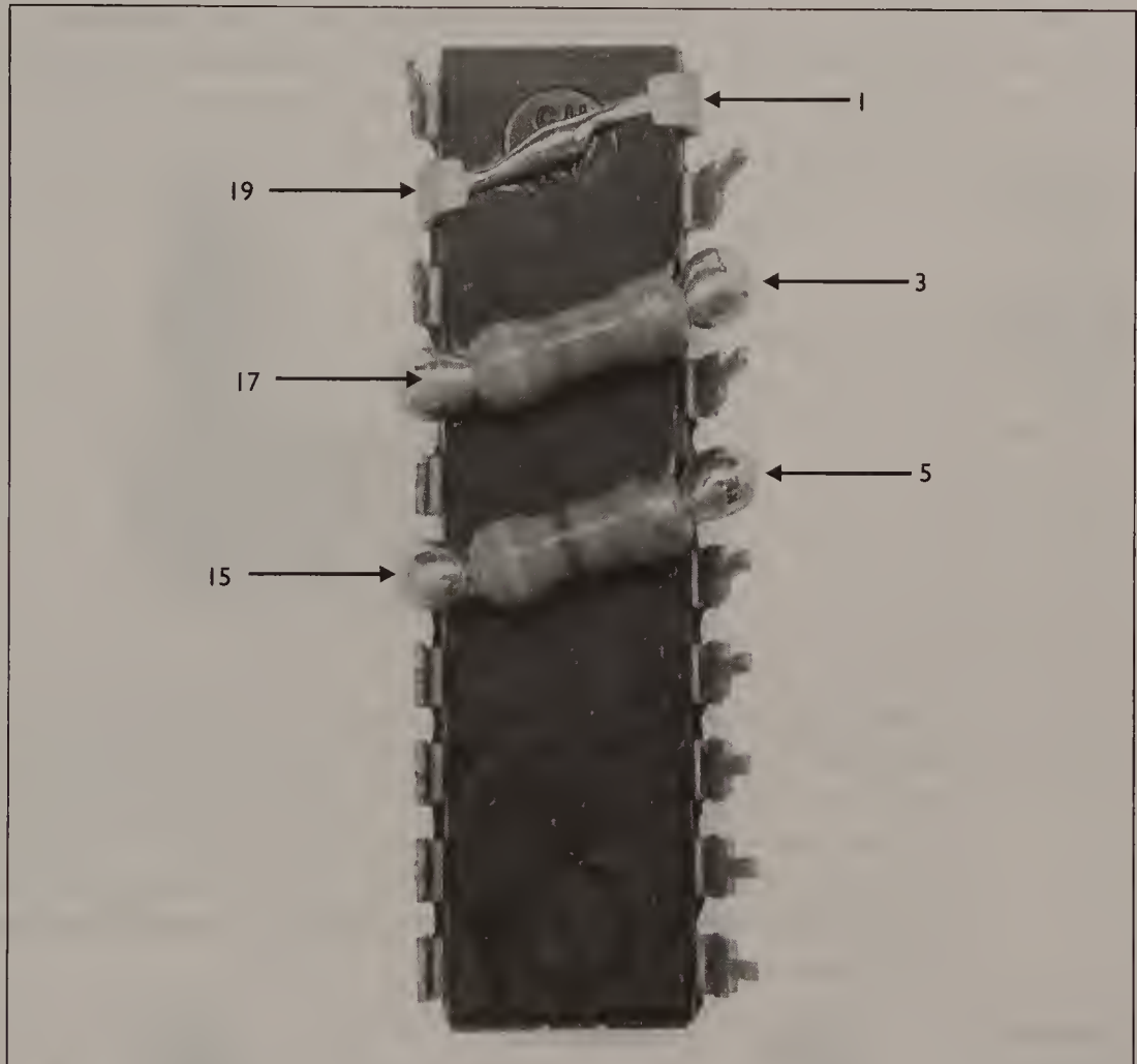
Figure 13-19 IMx free- forming: Adding the 47k resistors, and tying the enable lines together
