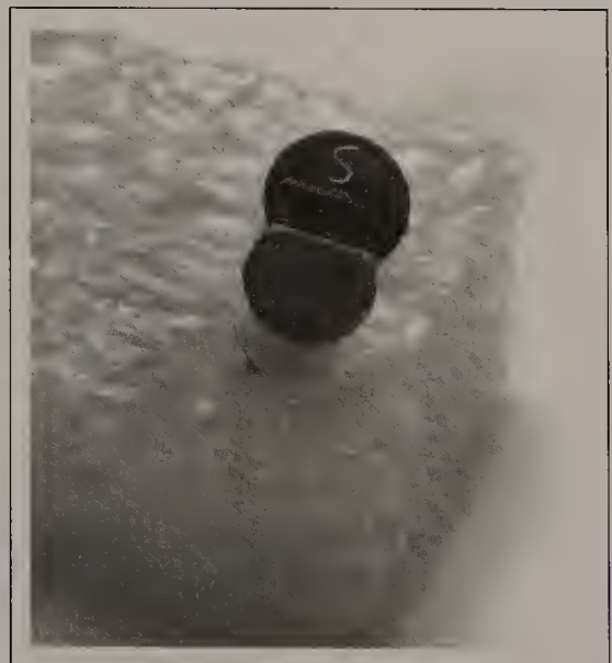
Figure 8-6 The larger one with the S is a 1381-S trigger.
