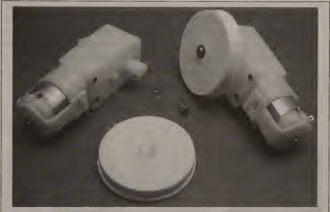
Figure 12-13 Mounting wheels to motors with screws and washers
