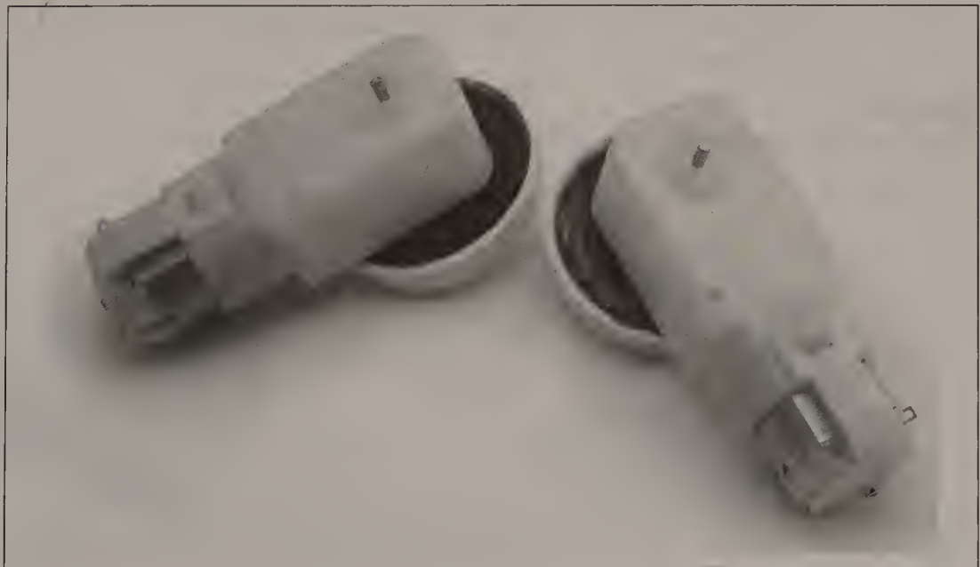
Figure 12-14 Filling the wheel cavities with epoxy
