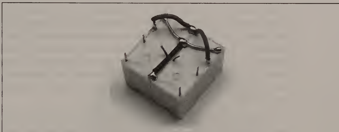
Figure 12-21 Wiring up the relay's "-" connections
