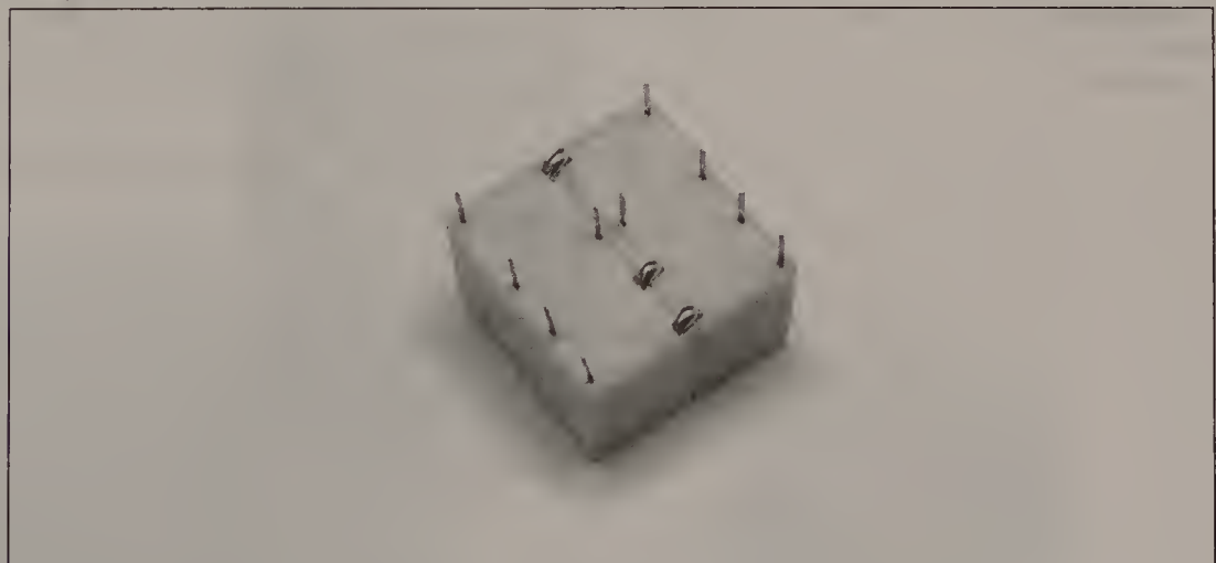
Figure 12-18 Soldering most of the middle row of relay pins
