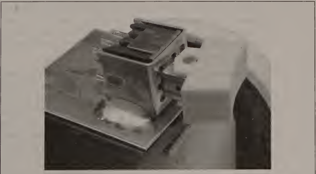
Figure 12-25 Soldering the switch to a holding plate and gluing the plate to the mini-sumo body
