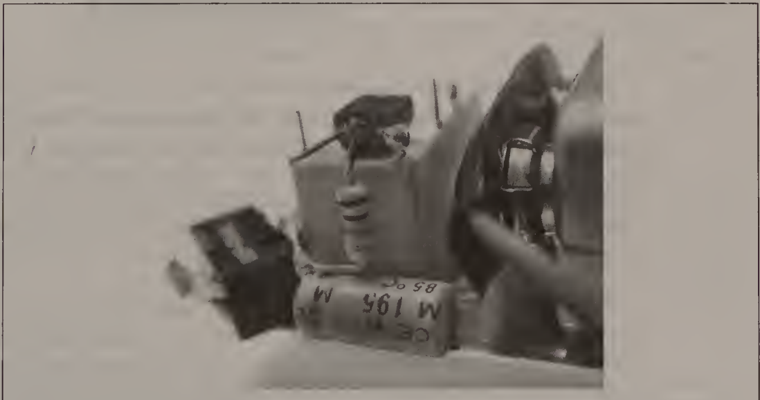
Figure 9-23 Installing the resistor across the capacitor and transistor
