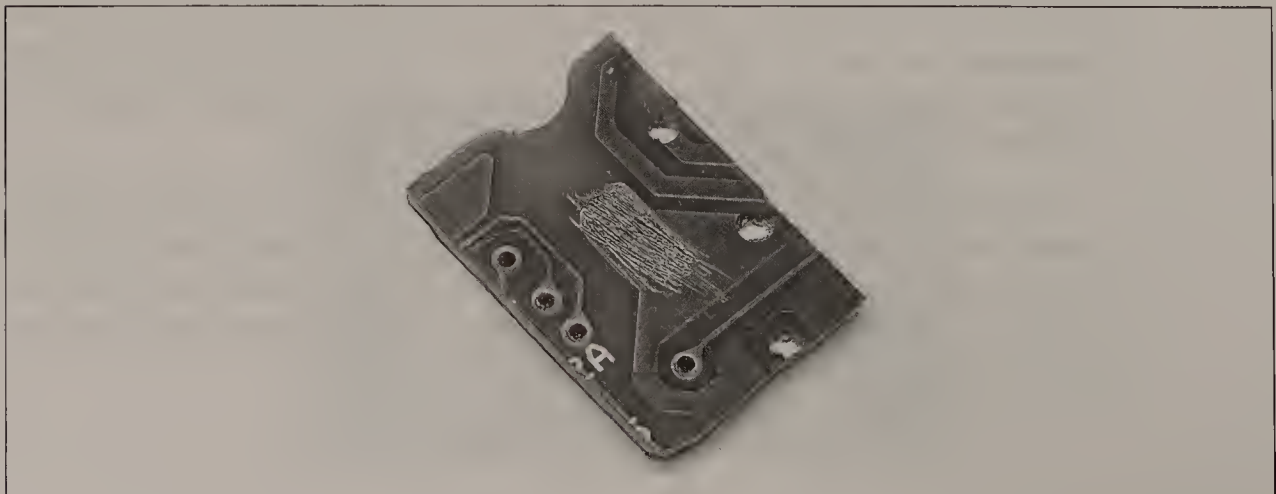
Figure II-23 Scrape off the masking to reveal the bare copper underneath.
