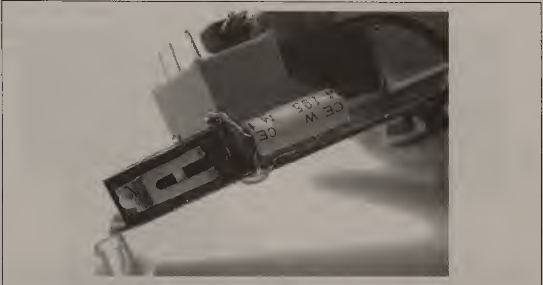
Figure 9-22 Soldering on the timer capacitor
