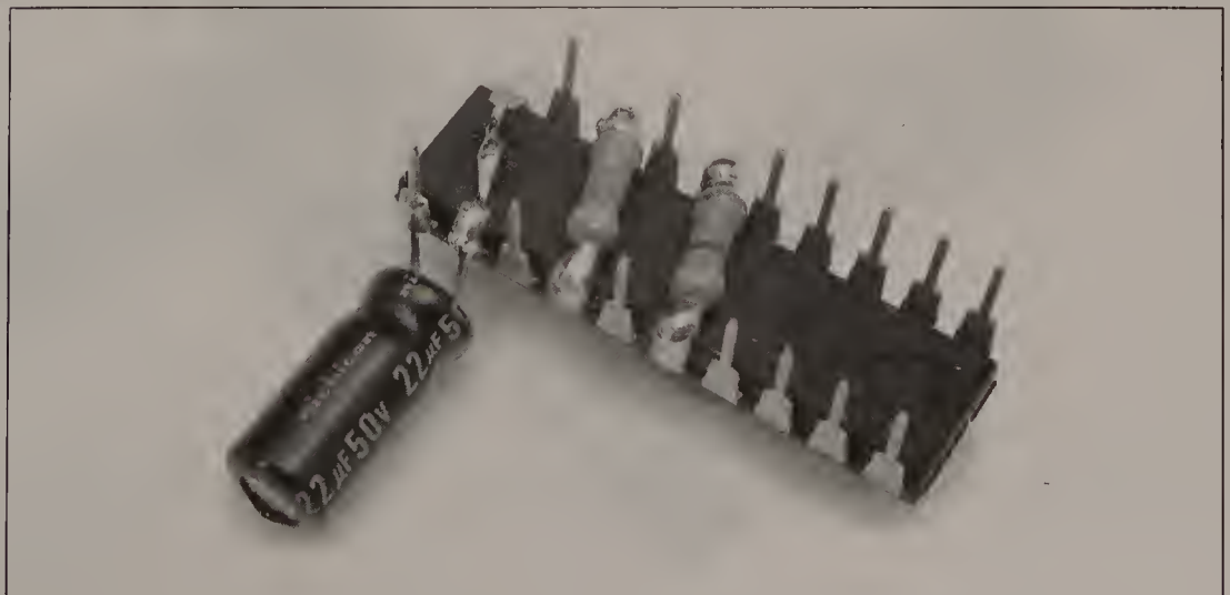
Figure 13-20 Soldering the 22 \mu F capacitor to pins 19 and 20
