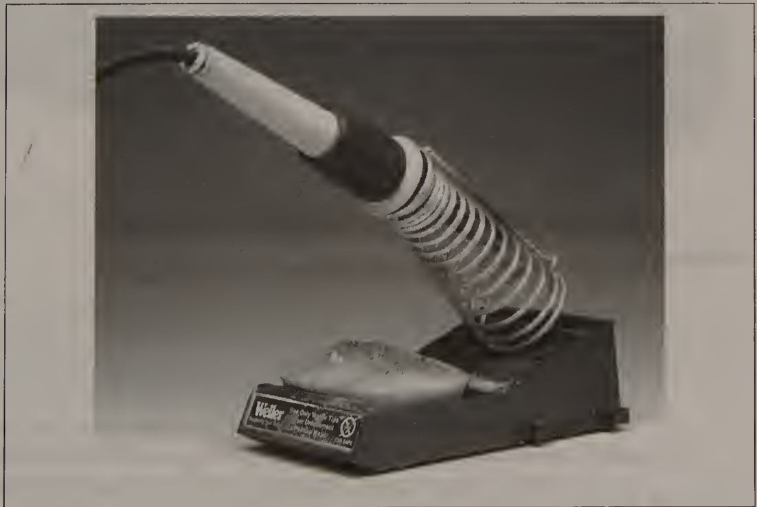
Figure 4-3 Don't mess with a 600°F chunk of metal on your desk; store soldering irons properly.
