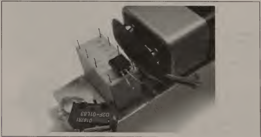
Figure 9-21 Mounting the relay, and soldering on the 2N3904/ PN2222 transistor
